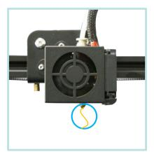
Press and hold the extruder lever then insert 1.75mm filament through the small hole of the extruder. Continue feeding until you see filament come out the nozzle.
